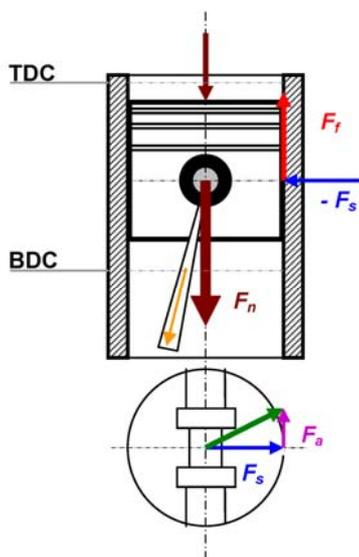
Fig. 1 Forces acting on the cylinder bore
