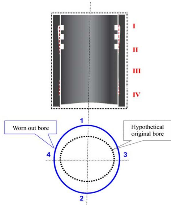
Fig. 8 Illustration of geometric deviations in the cylinder liner
