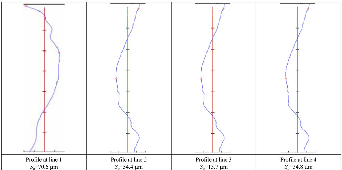
Fig. 7 Longitudinal sample profiles of cylinder straightness ( $S_a$  is the averaged straightness of the profile)
