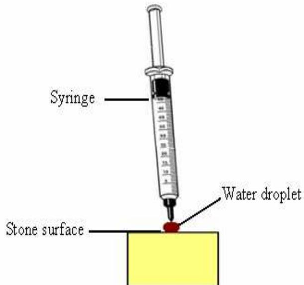
Fig.3. Method of stroking water droplet on the stone surface.
