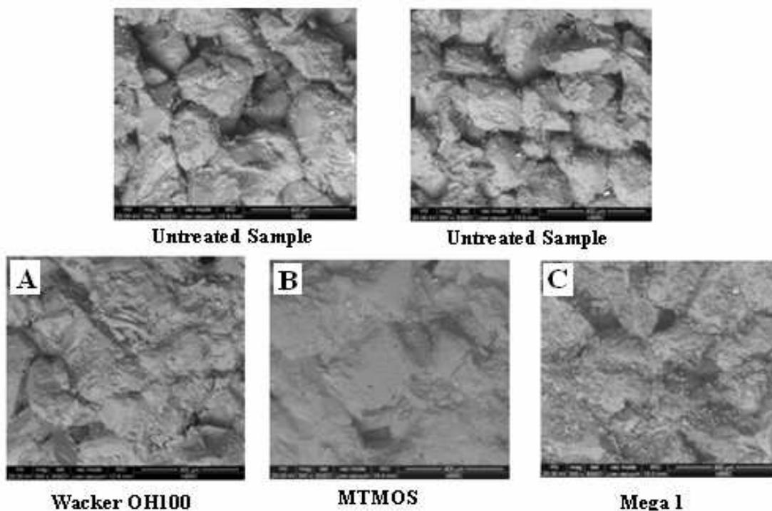
Fig.13. SEM micrographs of the treated and untreated sandstone samples.
