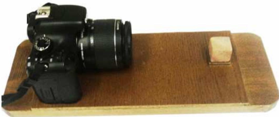
Fig.4. The method of capturing the images of static contact angle.
