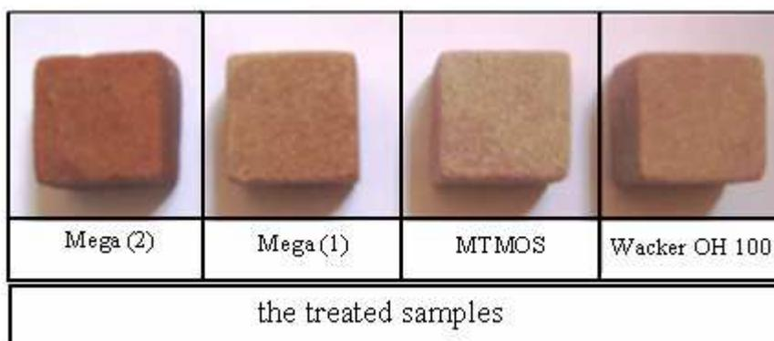
Fig .10. General appearance of the treated samples.
