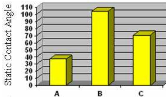
Fig .11. Results of static water contact angle of the treated sandstone samples.
