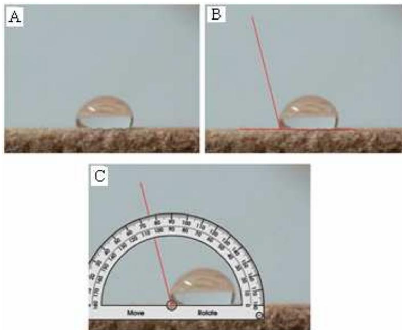
Fig.6. Manual calculation of the static contact angle by using a protractor.
