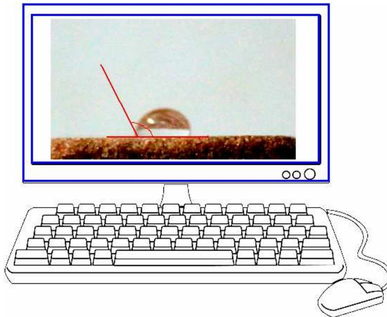
Fig.5. Automatic calculation of the static contact angle by using computer software program.
