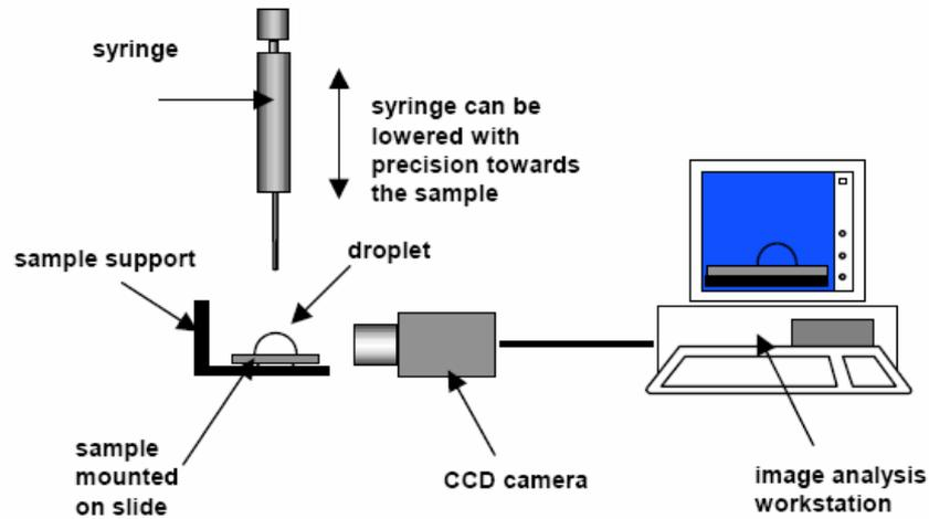
Fig.1. Components of the machines of static contact angle measurement.
