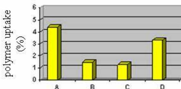
Fig.9. The values of polymer uptake by treated sandstone samples.
