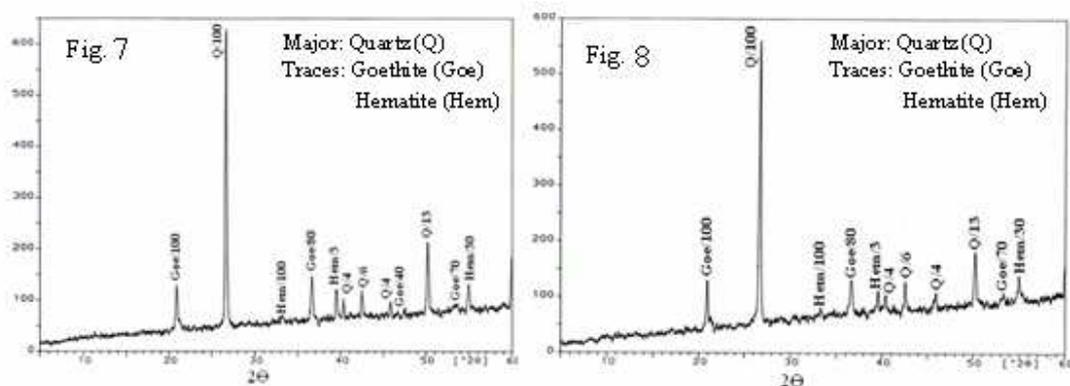
Figs. 7, 8. X-ray diffraction patterns of two sandstone samples.
